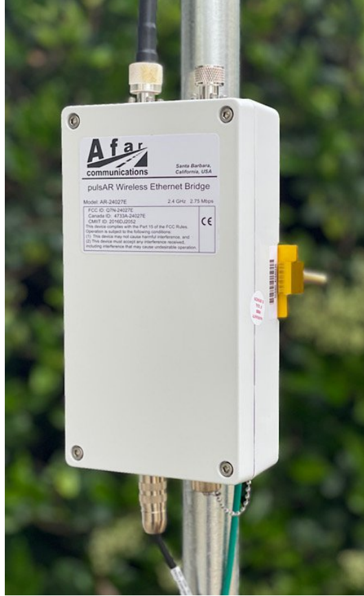
Figure 1.1: Pole Mounted Radio
